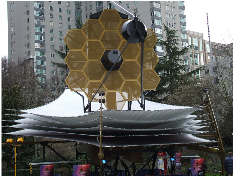
Figure 19: A mock-up of the James Webb telescope, displaying its five-layered sunshield.
